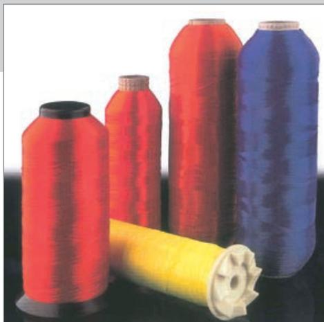
Continuous Filament Nomex yarn twisted to form an essentially round bundle. Material is available unbonded or bonded with a non-corrosive liquid nylon finish. Temperature range -55°C to 260°C, melting point 371°C.
