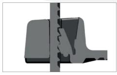
One-piece locking wedge provides consistent, reliable performance. Plus design offers low threading force reducing operator fatigue and improves productivity.
